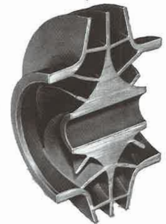
figure 4-30ab. vacuum casting process and section of a complex pump impeller vacuum cast in one piece (courtesy Aurora Metals Div. L.L.C.)
