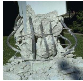
Kimmoton nurjahdus Inelastic buckling
