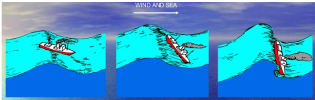
Figure 1.6. Stages of a Broaching to scenario : (a) The ship may run on crest; (b) ship stern gets too high and thus the rudder losses effect; (c) the bow pitches into trough and buries; (d) stern swings round bringing ship abeam to elements; (e) next wave will possibly break over the ship and cause severe damage.
