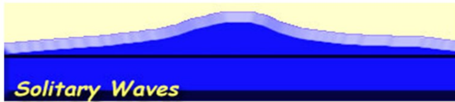
FIGURE 1. Schematic presentation of change in wave shape as wave advances into shallow water.
