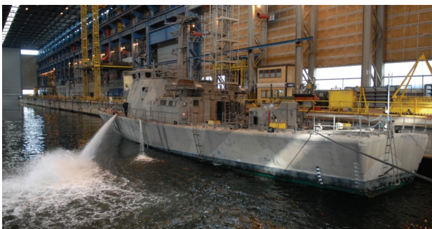
Figure 6: Pumping after a flooding test
