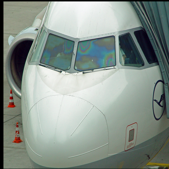
Indium Tin Oxide, ITO: Defrosting coating
