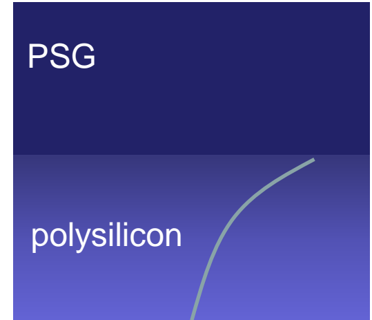
PSG (phosphorous doped silica glass) has doped polysilicon partially. PSG is homogenous, but polysilicon displays inhomogenous dopant concentration.
