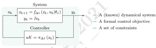
Find the best control sequence  $u_0, u_1, \ldots, u_{K-1}$  that optimally achieves the objective
