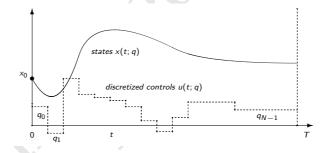
The idea is to discretise the controls u(t) on a fixed grid  $0 = t_0 < t_1 < \cdots < T_K = T$
