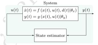
State estimation for use in control in the presence of sensor and model uncertainty
