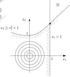
Continuity of the search domain and smoothness of the objective and constraint functions allow the use derivative-based approaches, applications of the Newton's method
