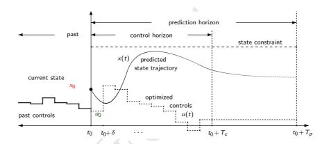
$$\min_{\substack{u_k, \dots, u_{k+N-1} \\ \forall n \in [k, k+N]}} \sum_{n=k}^{k+N-1} L(x_n, u_n) + L_f(x_{k+N}) \\ x_{n+1} = f_{\Delta t}(x_n, u_n, w_n | \theta_x), \\ x_n \in \mathcal{X}, \quad u_n \in \mathcal{U}, \\ \Phi(x_k, x_{k+N}) = 0,$$
