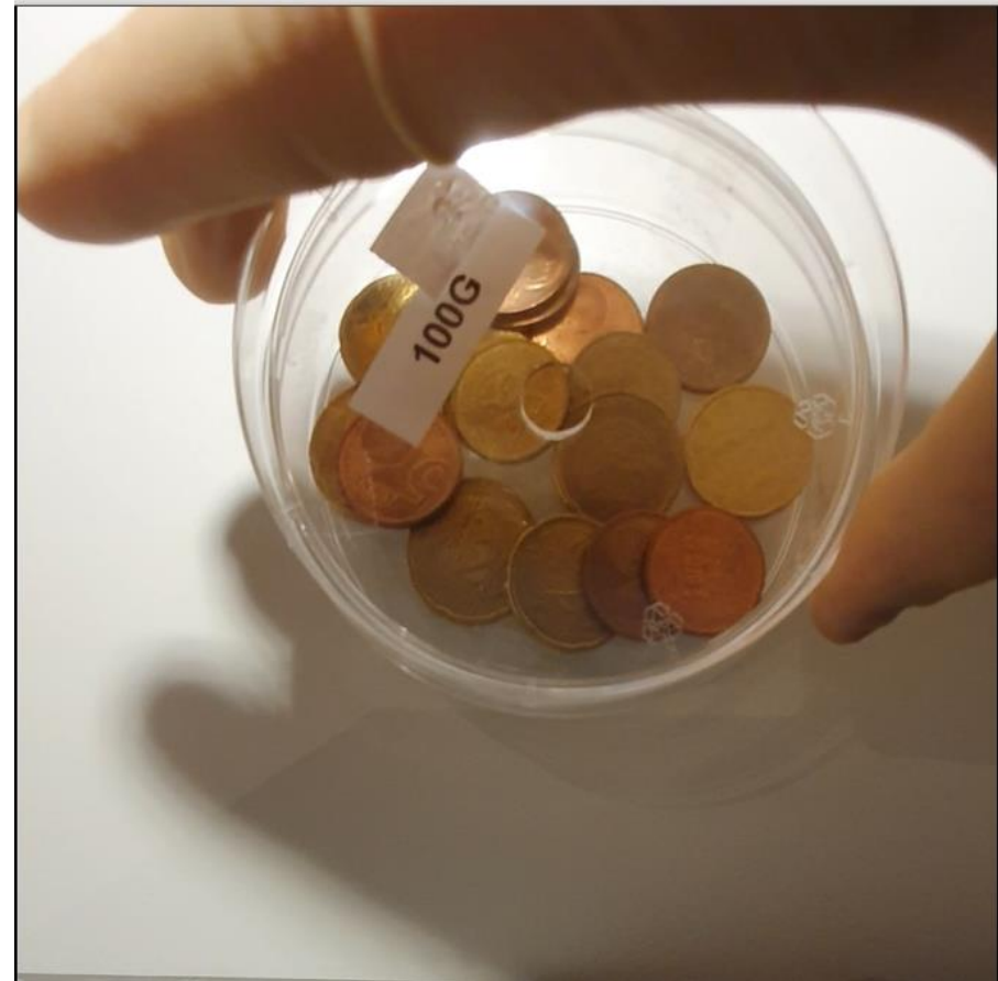
30:1 PDMS, 100 g weight, adhesion held
