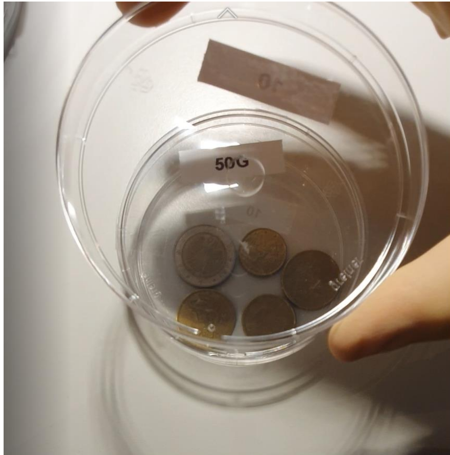
10:1 PDMS, 50 g weight, adhesion failed
