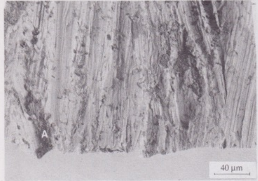
Fig 12 Scanning electron micrograph of the surface and cross section of a road grader blade worn against gravel. The surface has been damaged by chip formation, plastic deformation, and pickup of silica, revealed as dark, rough patches at A.
