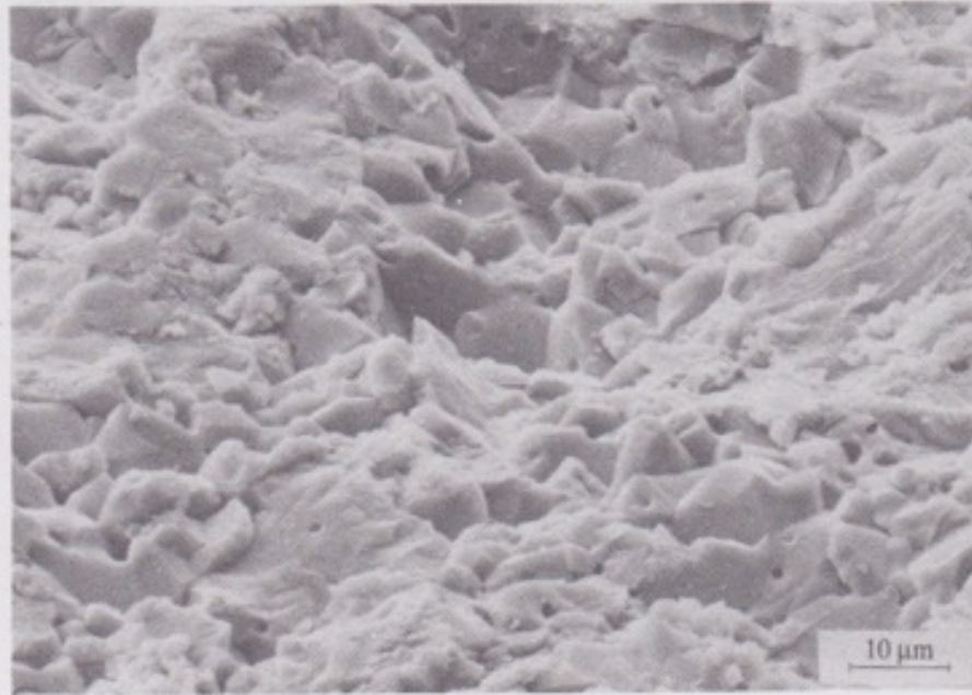
Fig 16 Scanning electron micrograph showing brittle fracture by particle erosion of an \text{Al}_2\text{O}_3 surface (250 \mu\text{m} SiC particles, 70 m/s velocity, 90° angle of impingement). Courtesy of Mikael Olsson
