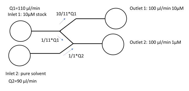
Figure 1: Example design that uses two inlets to make two dilutions. Make your drawing in a similar fashion. I used powerpoint, you can use whatever, including drawing by pen on paper and scanning/photographing.
