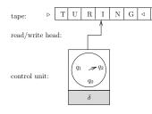
A finite state automaton with an unbounded tape that it can read, write, and move left/right one step at time.
