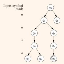
Now at least one computation path ends in an accept state when the input is fully processed, and thus the string *aaba* belongs to the language recognised by the automaton.
