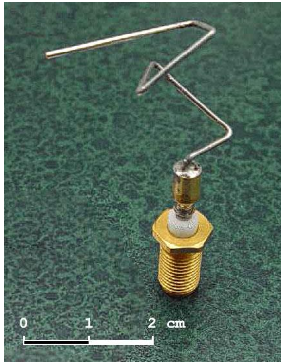
The 2006 NASA ST5 spacecraft antenna (Hornby et al., 2006)
