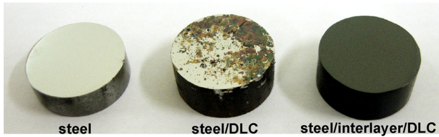
Fig. 7. Surface characteristics of the AISI 4140 plain steel polished (on the left), the AISI 4140 plain steel coated with DLC film without any adhesion interlayer (on the middle) and the AISI 4140 plain steel coated with DLC film in the presence of the a-SiC x :H adhesion interlayer deposited at 673 K for 10 min (on the right).
