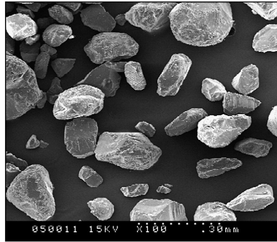
Fig. 2. SEM micrograph of the SiC abrasives used for erosion tests.
