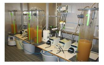
Sequencing Batch Reactors (SBRs) with operating volumes of 12 litres are operated in temperaturecontrolled chamber at  $14\pm1^{\circ}$ C ( $8\pm1^{\circ}$ C for Group 4). Feeding with synthetic wastewater during feeding sequence is done by peristaltic pumps with flow rate of 6 l/d. Fine bubble aerator is placed in the bottom of the reactors for constant aeration (2-3 l min<sup>-1</sup>). The SBR reactor is operated with an SRT of 12 days.
