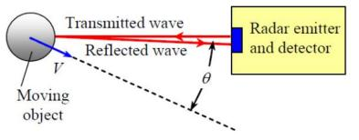
Working principle of radar velocitimeter:
