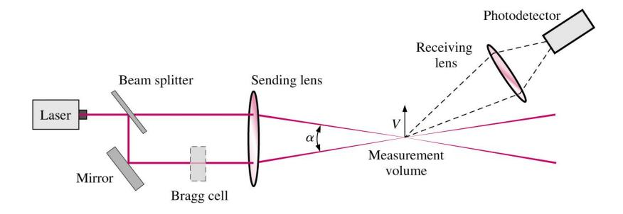
LDV is used to measure the velocity of particles in the fluid
