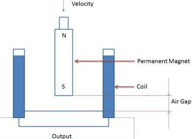
• Polarity of voltage determines the direction of motion
