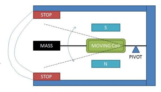
• These transducers are used for measuring velocities in linear, sinusoidal or random manner.
