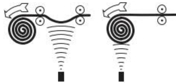
Figure 15.1.25: Two ultrasonic sensors provide roll diameter and tension control by providing outputs directly proportional to distance and roll diameter.
