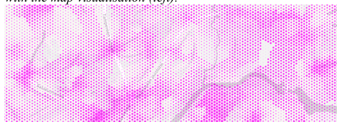
Figure 2. Fragment of the regular grid of points used for the calculation. Weight values are visualised as the diameter of every point.
