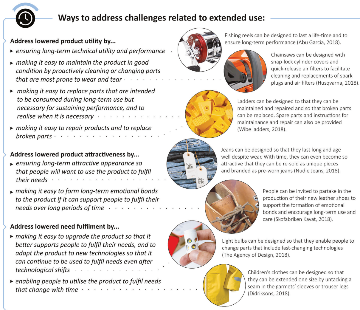
Fig. 7. Examples of ways to enable extended product use and make this more appealing. Product and service examples provided by Abu Garcia (2018), Husqvarna (2018), Wibe ladders (2018), Nudie Jeans (2018), Skofabriken Kavat (2018), The Agency of Design (2018), and Didriksons (2018).
