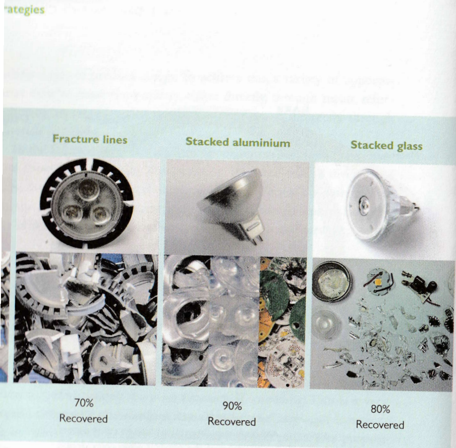
Figure 5. A LED spot light (top left) and three redesigns employing different materials and connections to improve the recycling result. The images at the bottom show typical fragments resulting from a shredding test. Recovered fractions are given in weight-%.
