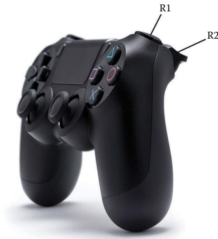
Figure 8.5 Every game controller has a unique set of design considerations, such as the varied responsiveness between the L1/R1 and L2/R2 shoulder buttons on the PlayStation DualShock 4 controller—determining which buttons are assigned to certain actions.
