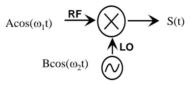
$S(t) = A\cos(\omega_{1}t)B\cos(\omega_{2}t) = \frac{AB}{2}(\cos(\omega_{1}-\omega_{2})t + \cos(\omega_{1}+\omega_{2})t)$ down-conversion
