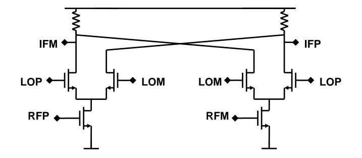
Independent RF transistors have poor matching
