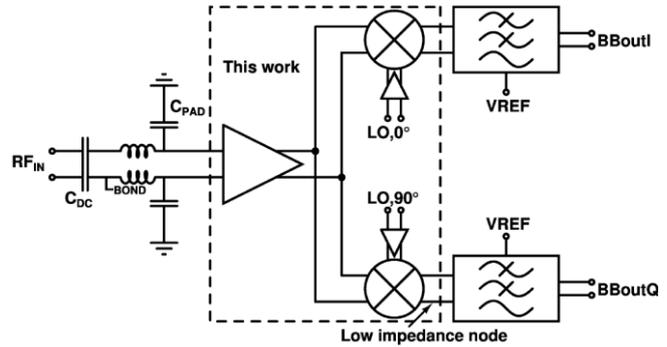
Figure 1. Block level details of the project work.
