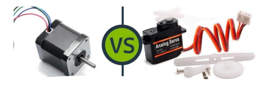
**Servos** have a limited range, i.e., cannot turn very long into one direction before stopping. **Steppers** can run continuously, so, you can, e.g., use them to drive continuous wheels.
