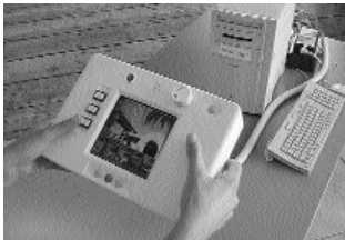
Figure 7: To communicate selected experiential aspects of the design concept for a digital camera, this prototype sacrificed appearance, weight and scale. Instead the effect of quality and speed of response of on-screen imagery on users' experiences were directly communicated to the audience members who were able to experience these dynamic behaviours themselves.
