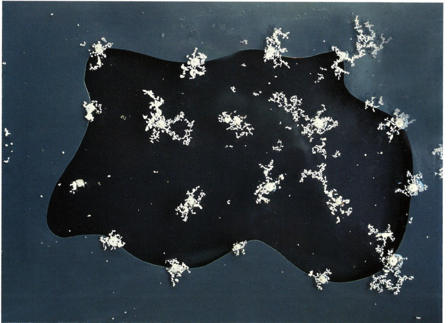
Frei Otto, occupation with simultaneous distancing and attracting forces, Institute for Lightweight Structures (ILEK), Stuttgart, Germany, 1992. Analogue models for the material computation of structural building forms (form-finding) are the hallmark of Frei Otto's research institute. The same methodology has been applied to his urban simulation work. The model shown integrates both distancing and attractive occupations by using polystyrene chips that cluster around the floating magnetic needles that maintain distance among themselves. © Frei Otto.
