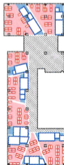
5 Automated "test fit" generates amenity rooms from space matrix and desk layout.
