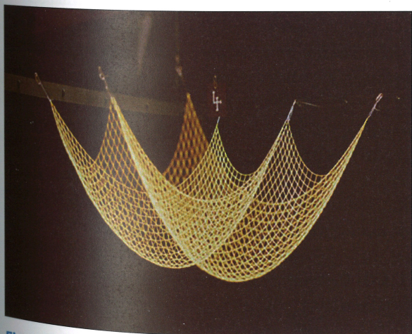
Figure 5.3 Hanging model experiments from IL
