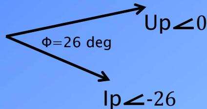
$$S = 3 U_P I_P^* = 3 * 230 < 0^\circ * 10 < 26^\circ \text{ VA} = 6.9 < 26^\circ \text{ kVA}$$
