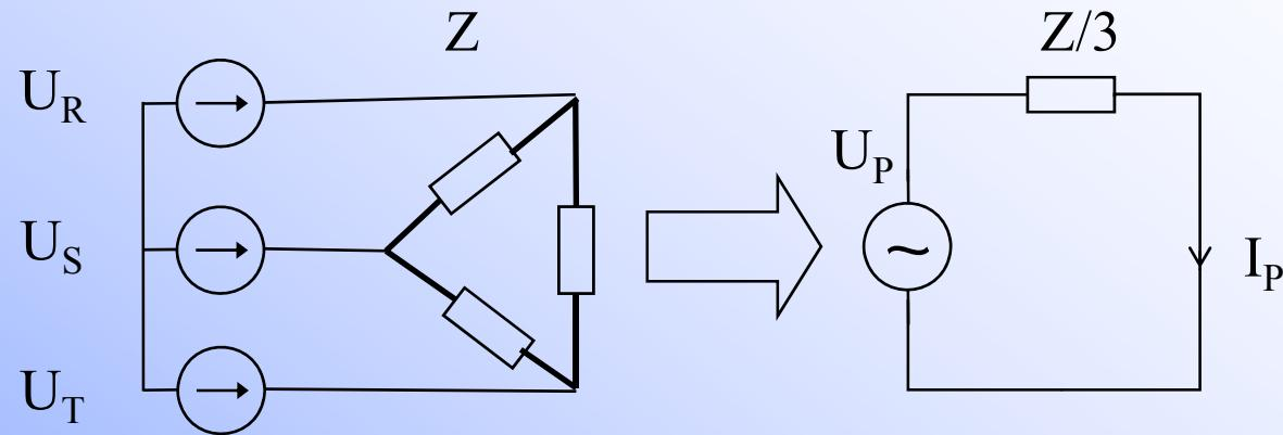
In three phase systems, the analytical solutions are made using single line diagrams where impedances are between phase and neutral, i.e. in star
