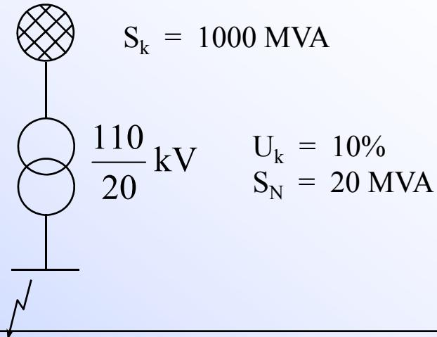
$$X_k = \frac{U_1^2}{S_k} = \frac{110^2}{1000} = 12,1 \Omega \quad (110 \text{ kV})$$
