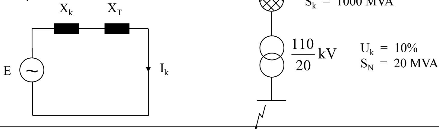
$$X_k = \frac{U_1^2}{S_k} = \frac{110^2}{1000} = 12,1 \Omega \quad (110 \text{ kV})$$
