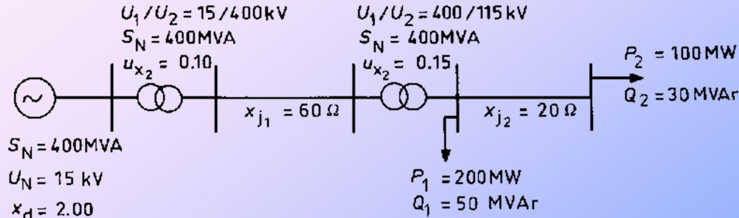
$$S_b = 400 \text{ MVA} \quad \& \quad U_b = 400 \text{ kV}$$
