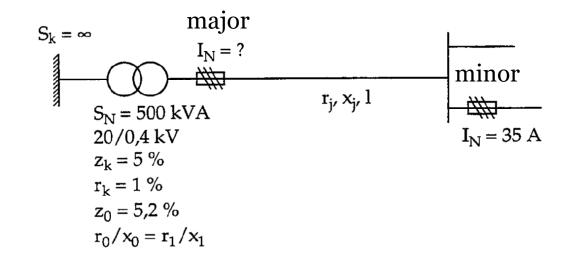
Choose the smallest possible fuse to the transformer's low-voltage side so that the protection is selective considering the  $I_N = 35$  A fuse. The two cases are:
