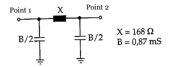
10 MW of active power is transferred using a three-phase line shown in the picture. Line-to-line voltages in the both ends of the line are 110 kV. **Calculate the power factor (cos\phi) of the load.**
