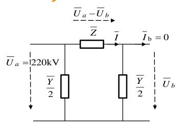
$$\overline{Z} = (r+j\omega l)s = (r+jx)s = \left(0.07\frac{\Omega}{\mathrm{km}} + j0.32\frac{\Omega}{\mathrm{km}}\right)200\mathrm{km} = 65.51\angle77.66^{\circ}\Omega$$
