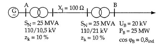
• Calculate per-unit values for all the parameters in the picture above. Use base values:  $S_b=50$  MVA and  $U_b=110$  kV
