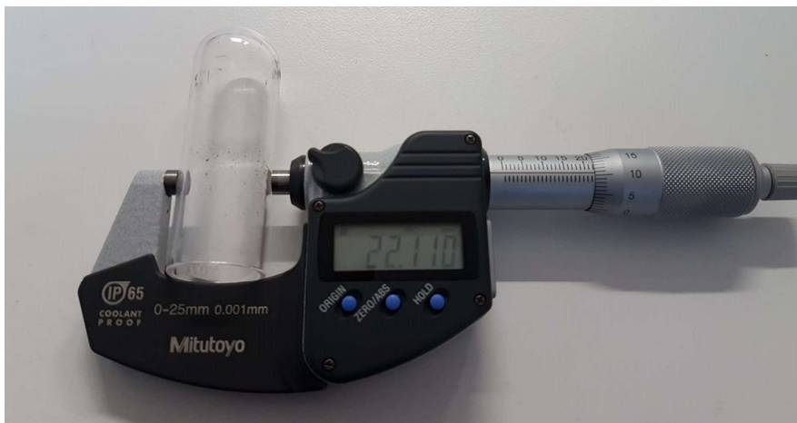
Figure 7 Cylinder outer diameter measurement
