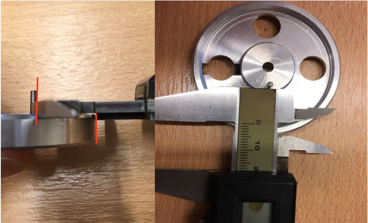
Figure 12 Pin location measurement
