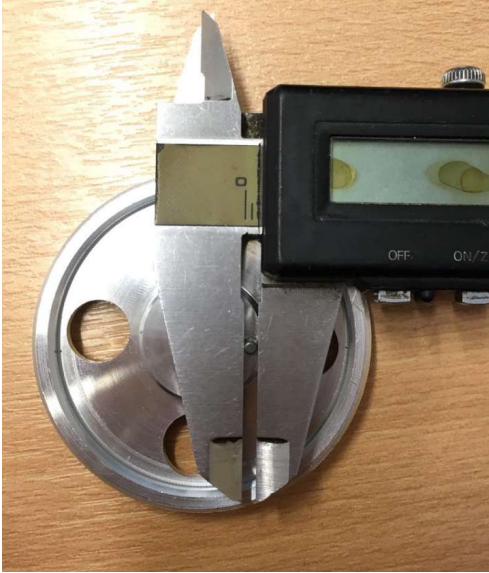
Figure 13 Pin diameter measurement
