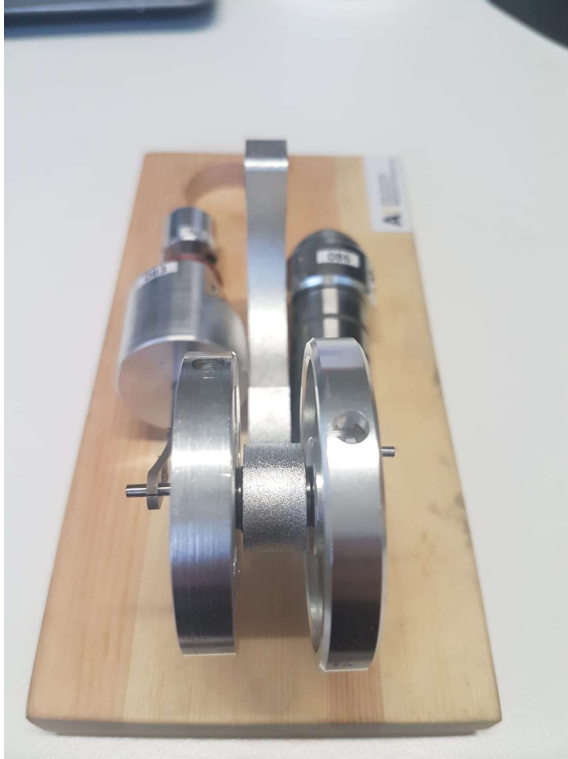
Figure 18 Flywheels, displacer piston, and power piston assembly.
