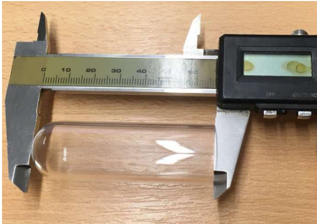
Figure 8 Cylinder length measurement
