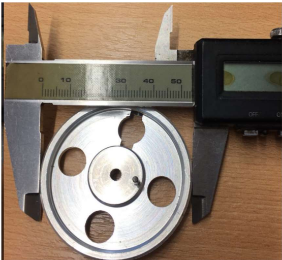
Figure 14 Flywheel diameter measurement
