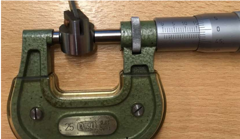
Figure 10 Power Piston diameter measurement
