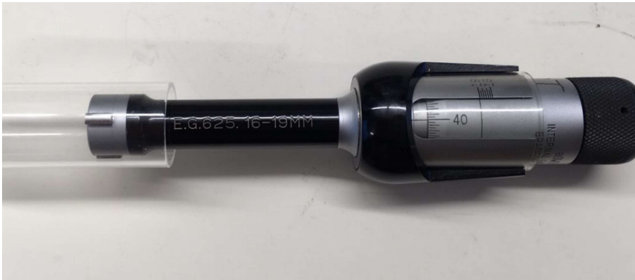
Figure 6 Cylinder diameter measurement
