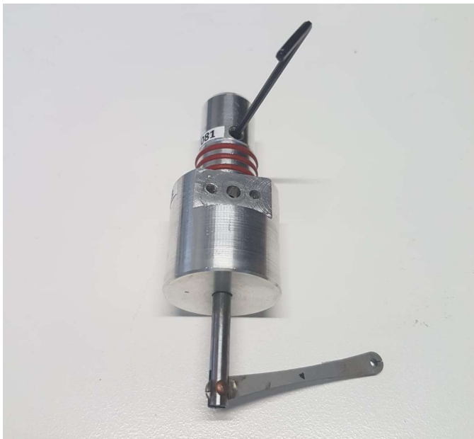
Figure 17 Displacer piston assembly.
