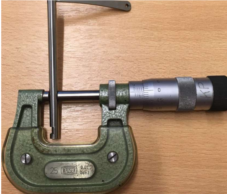
Figure 9 Micrometer measurement of displacer rod diameter
