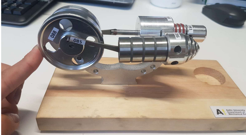
Figure 20 Flywheels, displacer piston, and power piston assembly.
