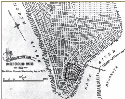
figure 1. Map of lower Manhattan showing the original area served by the Pearl Street station and its distribution system (courtesy of the Consolidated Edison Company of New York).
