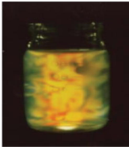
Photograph of liquid crystal suspension of cellulose nanocrystals
