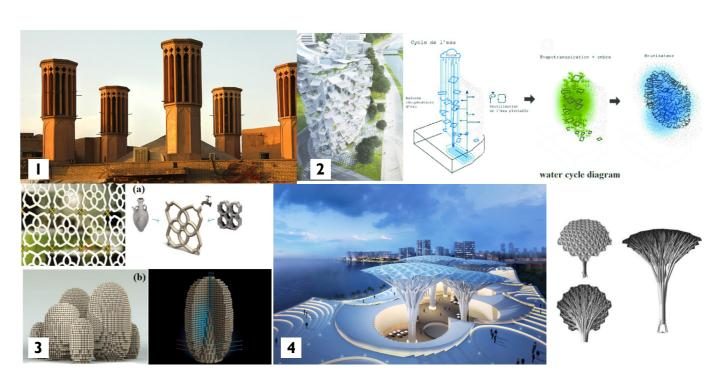
1; Windcatcher: a traditional architectural element used to create natural ventilation and passive cooling in buildings., 2; L'Arbre Blanc nature-inspired tower and its water cycle diagram (photo credit: Sou Fujimoto Architects, Nicolas Laisne Associes, and Manal Rachdi OXO Architects), 3; (a) E-cooler and (b) 3D printed pods concepts (photo credit: Andrew Michler), 4; Tree-shaped canopy design (photo credit: Iñaki Ábalos and Renata Sentkiewicz),
