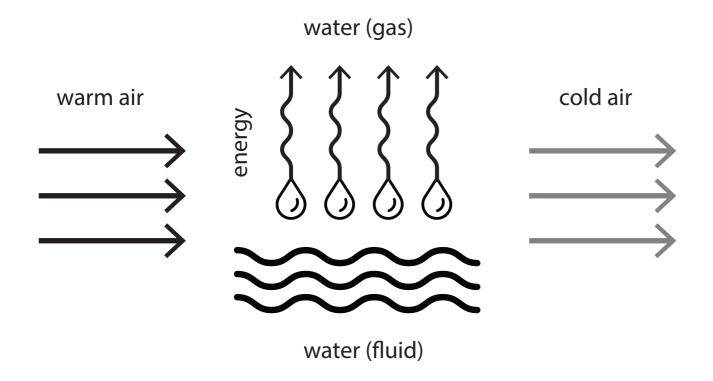
The heat exchange between the air and cooling medium can be direct or indirect. Direct evaporative cooling systems rely on the direct channeling of water into the airflow, while in indirect systems the primary air is cooled but no moisture is added into the air, which can play an important role in building air-conditioning systems. The disadvantage of indirect evaporative cooling technology lies in its high dependency on ambient air conditions.
