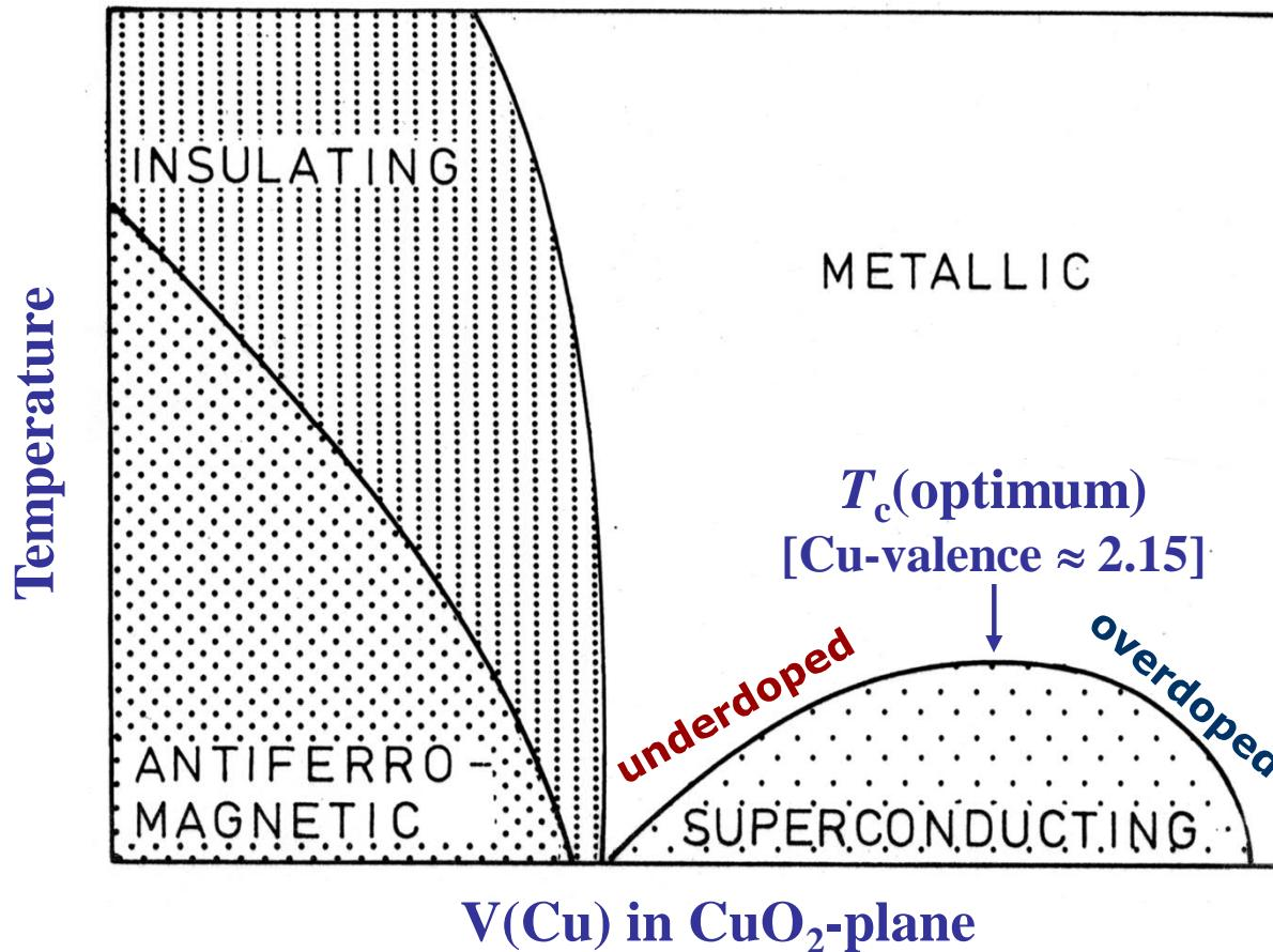
Oxygen content in  $\text{YBa}_2\text{Cu}_3\text{O}_{7-\delta}$  controls the valence state of copper, and thereby the superconductivity ( $T_c$  value)
