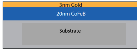
Figure 11: A side-view of the sample which will be used during these experiments. A 20nm CoFeB film is grown on to the Si substrate. 3nm Gold caps the sample
