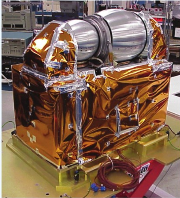
Figure 9-31: The Advanced Technology Microwave Sounder (ATMS) ready for integration on the Suomi NPP satellite. The sensor dimensions are 70 \times 60 \times 40 cm and mass is 74.1 kg. [Courtesy of Northrop Grumman Electronic Systems.]
