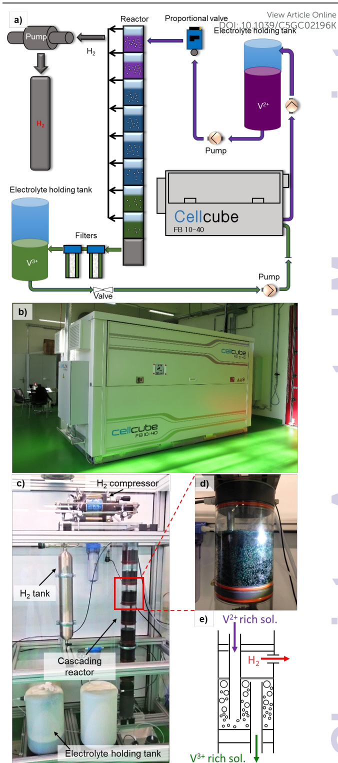
Figure 3. a) The flow diagram of the hydrogen reactor part of the demonstrator. b) The demonstrator is based around a 10 kW / 40 kWh all-vanadium flow battery which was retrofitted with c) an auxiliary hydraulic circuit for producing hydrogen. d) The reactor contains eight identical stages, where e) electrolyte is injected at the bottom of each stage and flows upward through the catalytic bed before reaching the outlet down to the next stage. Hydrogen is collected from the head-space of each section and compressed into the storage tank.
