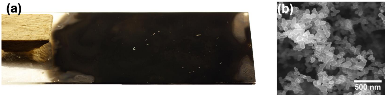
Figure 6: a) Superhydrophobic soot surface with some defects (little white marks and reflective areas near the edges). b) Scanning electron microscope image of the coating showing the nanoporous soot structure (reproduced from 5 ).
