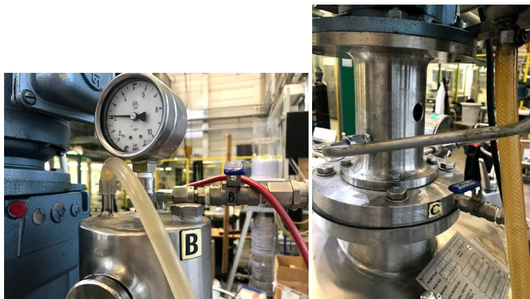
Figure 2. Outflow valve (B) and pressure meter and input valve (C) into stirrer motor shaft seal.
