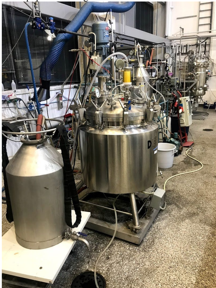
Figure 1. Usage in which air-pressure is used drive sugar medium liquor to the bioreactor from mixing tank Diessel
