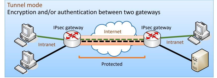
Gateway routers establish the IPsec tunnel; routing rules send traffic through the tunnel
