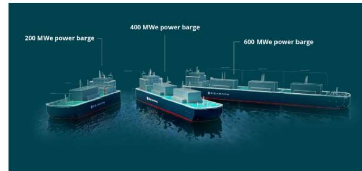
Seaborg is planning three variations of its molten fluoride salt reactors Image Credit: Seaborg Technology
