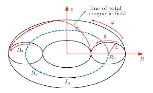
Toroidal angle:  $\varphi$  Poloidal angle:  $\theta$  Toroidal field:  $B_{\varphi}$  Poloidal field:  $B_{\theta}$  Major radius: R
