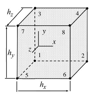
Bi-linear and tri-linear shape functions of 2D and 3D cases are products of the linear shape functions of the 1D case.
