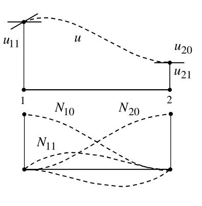
In xz-plane bending  $u = u_z$  and  $du / dx = -\theta_y$ , in xy-plane  $u = u_y$  and  $du / dx = \theta_z$ . Week 47-40 • In one-dimensional case, the brute force approach works. Let us collect the coefficients of the monomials of the shape functions into a matrix, and use the definition of the shape functions
