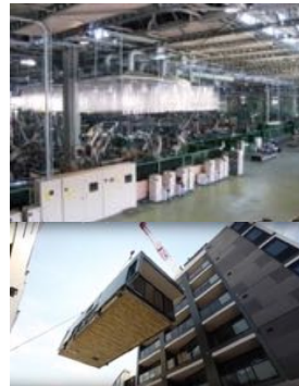
Automatized prefabrication of building modules
