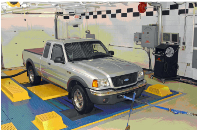
Fig. 12.4 The 4×4 Vehicle Chassis Dynamometer with individual wheel control
