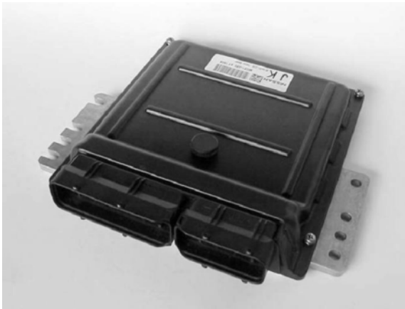
Fig. 6.6 A typical 'black box' Engine Control Unit (ECU) module
