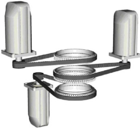
Fig. 5.6 Servo motor controlled patterning mechanism
