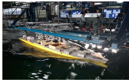
Figure 0-8 Model testing remains key part for the validation of ship dynamics of novel hull forms
